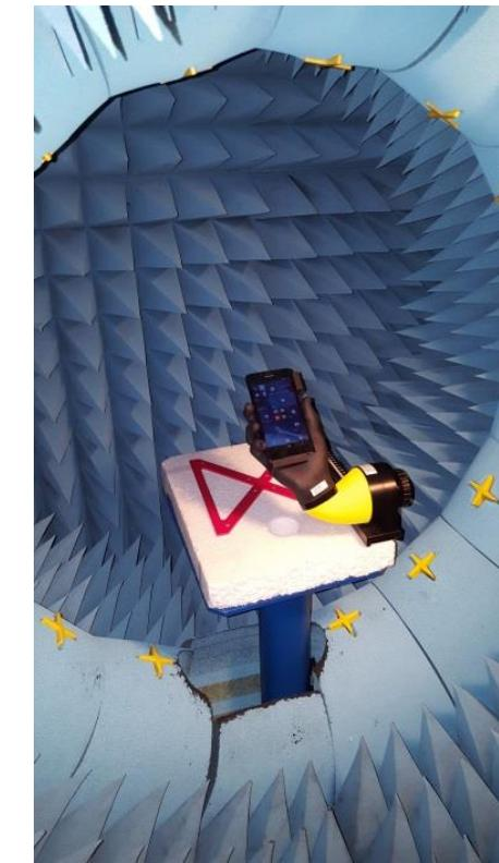
*Setup for voice and data services including the specified phantom. All phantoms are as specified in the CTIA test plan [CTIA15] and made by Speag AG.*
