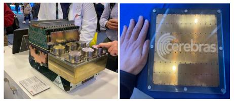
Multiple Cerebras nodes are interconnected into a cluster setup where 12x100 Gb ethernet connects deliver an aggregated interconnect bandwidth of 1200 Gb/s. Each node is cased in a standard 15u rack.
