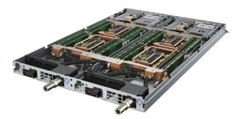
Liquid cooling solutions can remove from about 60% and up to 90% of all generated heat from a server, making the best solutions almost heat-neutral to the server room.
